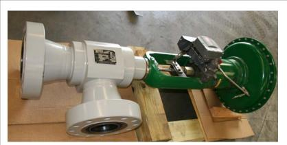
5-1/8"-API 10,000 psig, full 3.00" orifice with pneumatic diaphragm actuator
