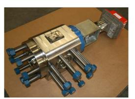
3-1/16"-15M all Nickel Alloys, "HH", PSL 3G (extra long 718 inlet studs for instrument flange)
