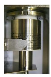
Stainless steel indicator drum. With markings to the nearest 0.0001 in., it is easy to read and remains in place when mounting rotary style electric actuators.
