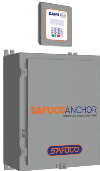
The Anchor ESD system is a self-contained autonomous emergency shutdown system for wellhead wing and master valves equipped with pneumatic or hydraulic actuators. It includes a gate valve (any size), electrically-driven hydraulic pump and manifold actuator, and a Safety Automated Monitoring Instrument (SAMI), the industry's premiere computer control system.
