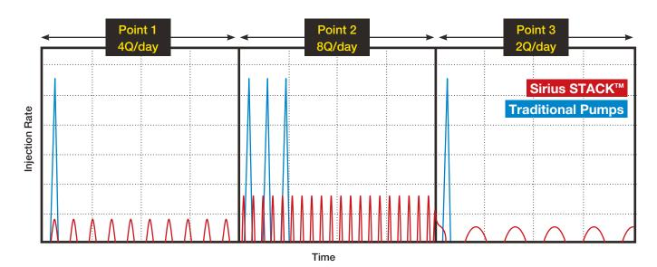
The Sirius pump speed varies between injection points depending on rates and cycle time required, which provides equal chemical contact time between points.
