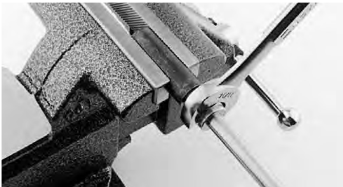
Place Pre-Set Tool in a vice and tighten nut specified number of turns
