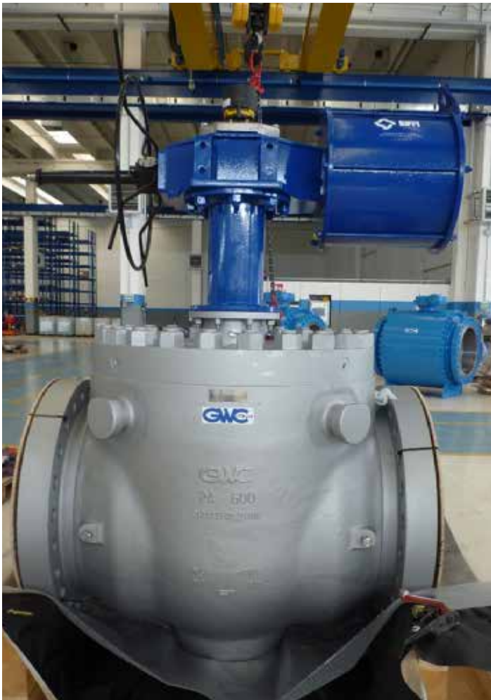
Pneumatic ESDV 24" Class 600 Top Entry
