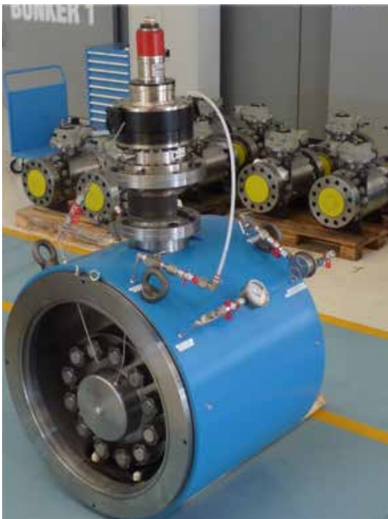
GWC Italia's R&D Dept. has designed and built its own Hyperbaric Test Chamber for Subsea Valves
