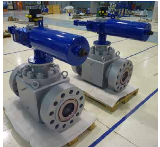
Pneumatic SDV 8" Class 600 Top Entry
